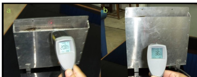
Figure 7. Figure showing the temperature of (a) the hot air coming out of the heater and (b) the front panel
