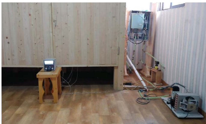
Figure 1. Experimental apparatus for natural convective radiative heat transfer cooling load for small cabins for one person
