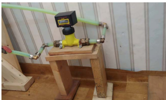
Figure 5. Flow measurement device for the cold water circulating inside the tube of cold water panels of the small cabin for one person
