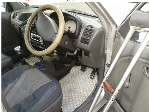
Figure 8: Connected assembly for the Accelerator and Break of the device 5
