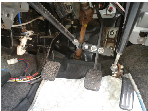
Figure 9: Reverse assembly of the break & accelerator of the device 5
