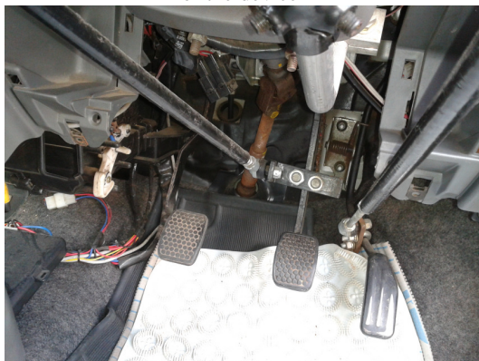
Figure 9: Reverse assembly of the break & accelerator of the device 5
