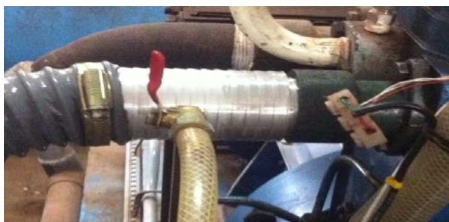
Figure 2. Carburetor for air and biogas mixing
