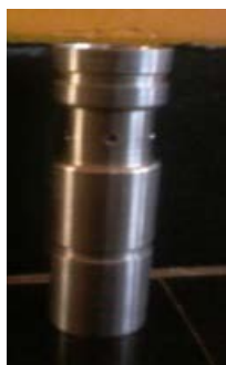
Figure 2. Carburetor for air and biogas mixing
