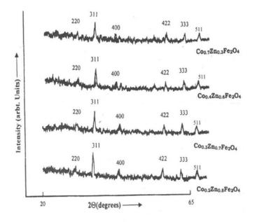
Figure 1..XRD Patterns of Co-Zn ferrites.
